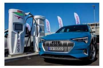
Figure 51 350kW ultra fast charger, Norway Source: CircleK
