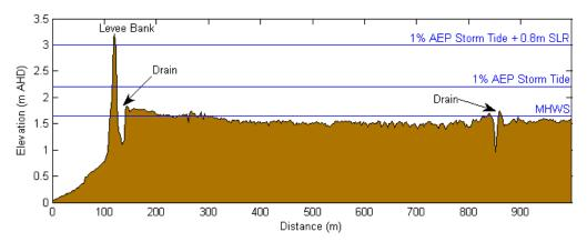
**Figure 3-2 Topographic Cross-section Extracted from the Terrestrial LiDAR Near Lang Lang.** The MHWS level is based on hydrodynamic modelling undertaken as part of this project and the 1% AEP Storm Tide level is from McInnes et. al., (2009).
