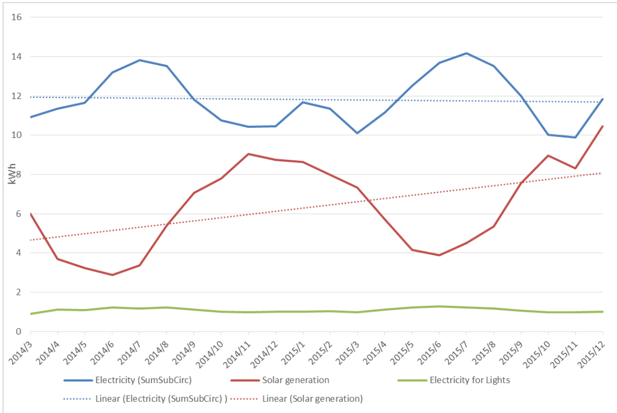
Figure 42: Monitored data average daily electricity consumption and generation by month and year
