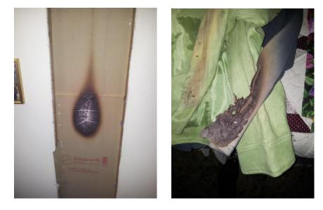
Figure 77: fire damage and burnt clothes found behind a faulty gas wall heater
